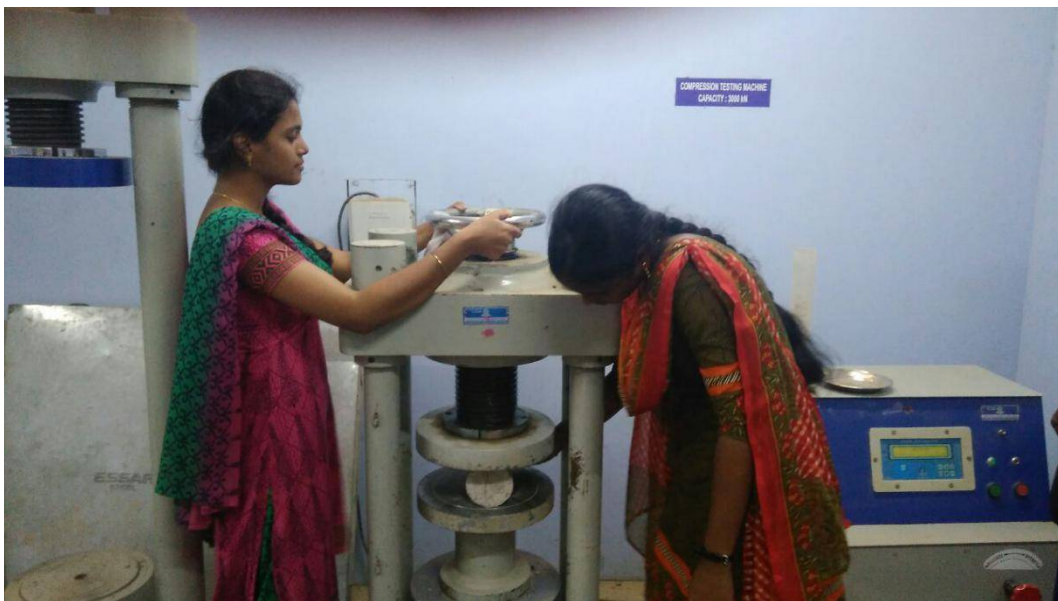
Fig 5.3 Test set up for split tensile test
